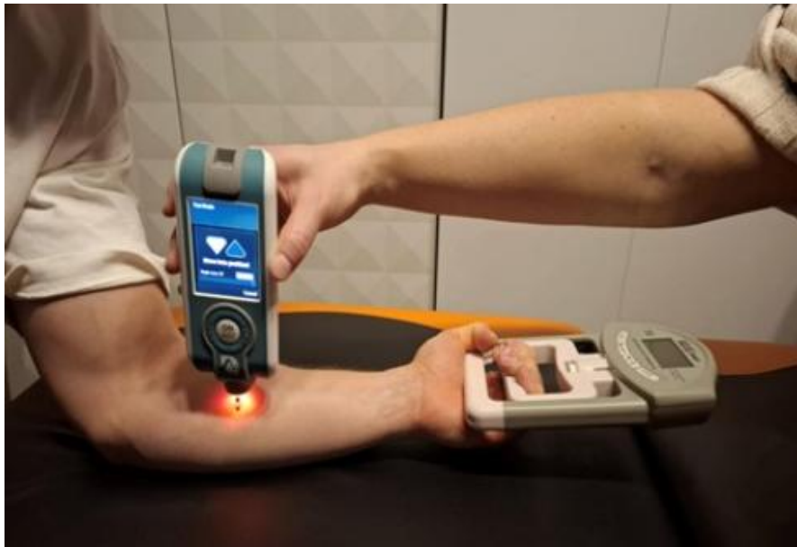
Figure 1. Muscle assessment under load using the Baseline handheld dynamometer and the MyotonPRO myotonometer.
